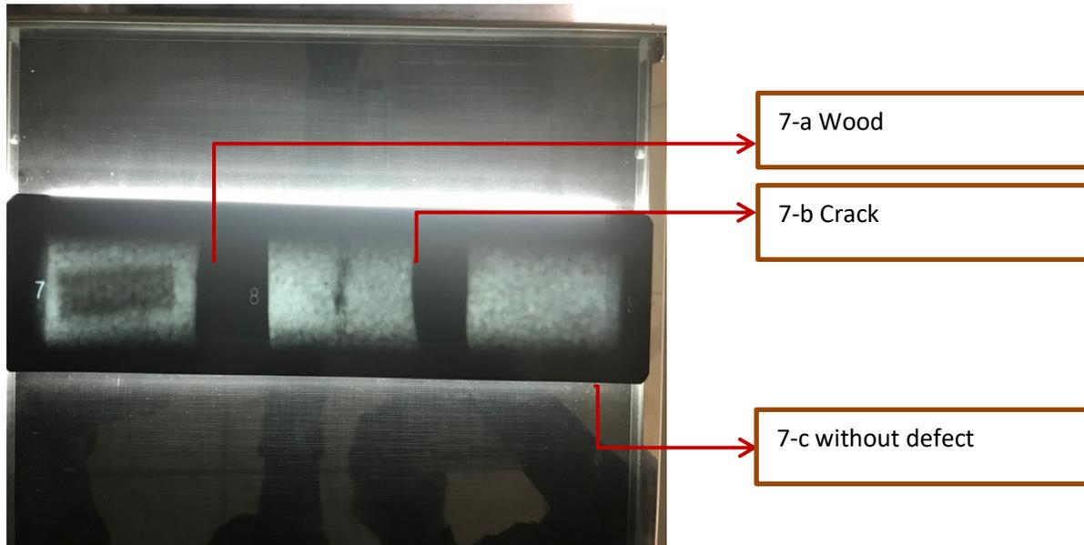
**Figure 7.** Image obtained by the radiography of samples n° 4, 5 and 9
