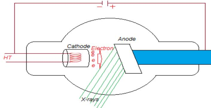
**Figure 2.** Basic x-ray production process
