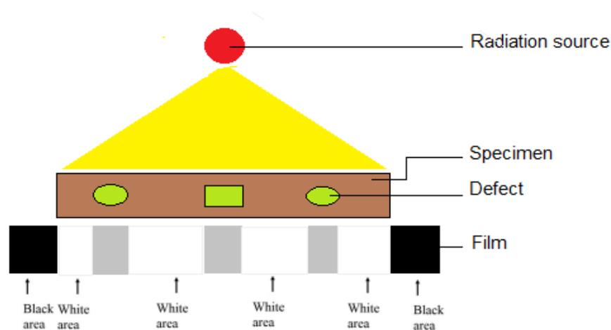
**Figure 1.** Schematic of radiography set-up
